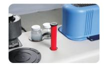
▶ If the red level indicator is raised at the upper part of the pre tank, replace the filter as it indicates that the filter is blocked.
